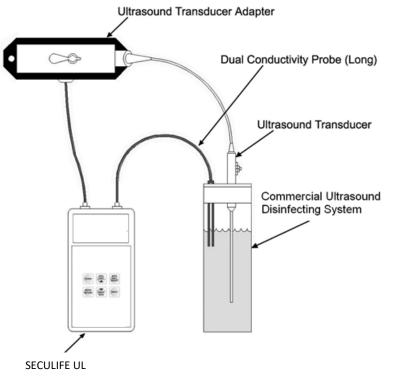
Typical Electrical Leakage Test
