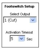
**Activate Footswitch** – This button is used to trigger the footswitch output for the duration that is configured in the Footswitch Setup menu. The footswitch can be deactivated before the activation timeout period by pressing the Activate Footswitch button a second time. While the footswitch output is active, the Activate Footswitch button will remain highlighted with a yellow background.
