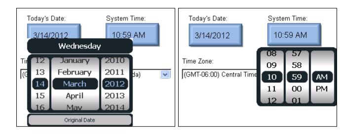
Then the Date/Time settings are set by scrolling the display to the desired value. Once the proper setting is shown, the Date/Time button is pressed again to accept the change.
