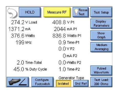
The above image shows typical measurements when "All Readings" is selected from "Display Parameters". The voltage, current, power, and time for each "pulse" is displayed, as well as the duty cycle for "pulse 1".
