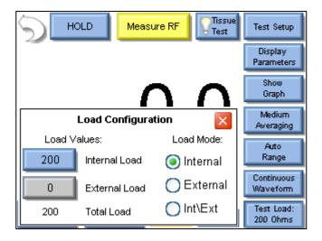
NOTE: The ES PRIME can be configured to use internal loads, external loads, or a combination of both. First select the Load Mode, then enter the desired internal and external loads. The total load will automatically be updated. For most testing, the internal loads will be sufficient.
