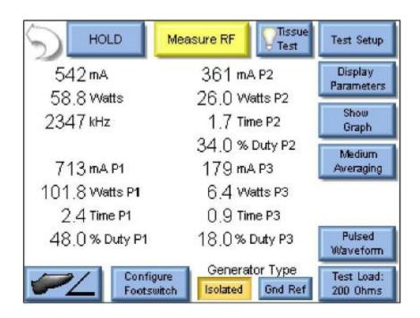
The above image shows typical measurements when "All Readings" is selected from "Display Parameters". The voltage, current, power, and time for each "pulse" is displayed, as well as the duty cycle for all three pulses.
