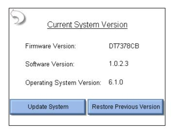
**Update System** – This button allows the user to update the ES PRIME through the internet (FTP site) or with a USB Flash drive.
