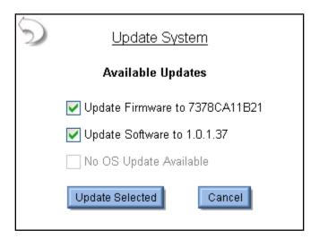
The user can perform all updates at once or select the software to update by using the check boxes. Once the desired updates are selected, the Update Selected button is pressed. The ES PRIME will automatically download and install the updates to the system. When updating the Software or OS, the ES PRIME will need to be rebooted.
