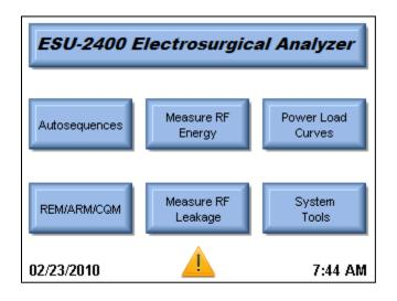
Pressing on the caution icon will display the active faults and the status of the faults. When a fault has been cleared, such as a blocked fan or system overtemp, pressing the Reset Cleared Faults button will remove the fault from the list. Once all faults are cleared, the caution icon will be removed from the main screen.
