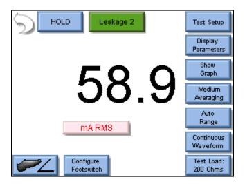
**Leakage Test 3** - I need to measure the leakage current from the dispersive (REM) port to ground. I need to have a 200 ohm load from Active to Ground during the test.
