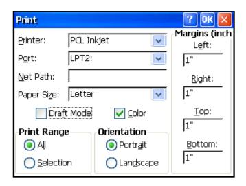
**Printer** – Select PCL Inkjet or PCL Laserjet based on the type of printer connected to the ES PRIME. Even if the printer name shows up in the list, i.e. OfficeJet H470, select the generic PCL Inkjet or Laserjet instead.
