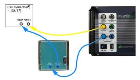
If the output terminals of the DUT are not compatible with the standard ES PRIME safety test leads, the alligator clips supplied with the ES PRIME accessory kit can be used to connect directly to the electrosurgical instrument as shown in the connection diagram below.
