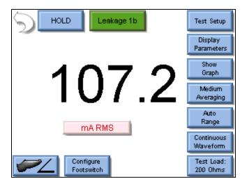
**Leakage Test 2**– I need to measure the leakage current from the dispersive (REM) port to ground. I need to have a 200 ohm load from Active to Dispersive during the test.
