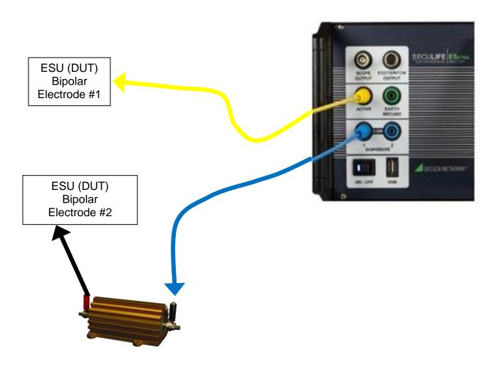
**Tissue Test -** This mode evaluates the tissue response function of the DUT. In this mode, the ES PRIME is configured for an external TRL-2420 lamp load. The ES PRIME is connected in series with the load as shown below. The terminals are labeled Return and Active for reference only. The DUT Return terminal shown below is typically not the Patient Return or REM electrode. Refer to the DUT service manual to determine which DUT ports are used for the tissue response output.
