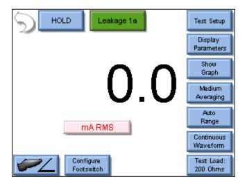
The buttons on this screen are described below in a clockwise sequence starting with the back arrow.
