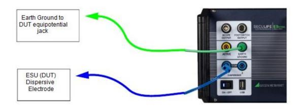
**Leakage 2** This leakage test, specified by the IEC as Earth Reference Leakage Type BF (Load Between Electrodes), is for testing the leakage to earth ground of a Ground Referenced Output type BF electrosurgical generator from the active output. This test complies with IEC 601.2.2, sec. 19.101a, test 1, fig. 102, and sec. 19.102, adopted by ANSI/AAMI HF18-2001. The purpose of this test is to verify that the RF leakage of the Device Under Test (DUT) meets or exceeds the IEC specification.
