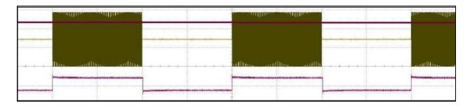
In the above illustration the purple line represents the user-selectable threshold. The signal at the bottom shows when the SECULIFE ES PRIME is taking a measurement of the waveform. Any time the waveform is below the threshold the SECULIFE ES PRIME considers it "off" and does not use that portion of the waveform for measurements
