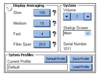
**Display Averaging** – The Display averaging settings of Slow, Medium, and Fast are programmed here. These determine the number of samples used in averaging the RMS measurements. The larger the number, the more stable the reading, but the less sensitive the system will be to small changes in readings. The filter span determines the maximum change in input readings that will be averaged.
