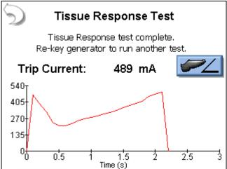
The Tissue Response Test will monitor the current in the load as the lamp heats up. When the current reaches the Tissue Response Trip point in the DUT, the generator output will automatically deactivate. At this point, the display will change to show the trip current as well as a graph of the current during the test. See page 11 for typical connections.
