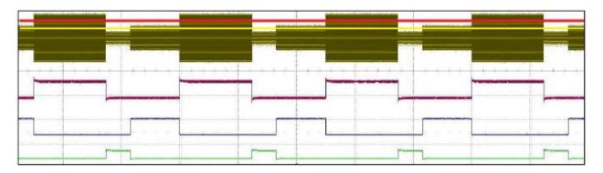
In the above illustration the red line represents the user-selectable threshold 1. The yellow line represents the user-selectable threshold 2. The purple signal represents when the waveform is above threshold 1 and the SECULIFE ES PRIME is measuring it as "pulse 1". The blue signal represents when the waveform is below threshold 1 but above threshold 2 and is being measured as "pulse 2". The bottom green signal represents when the waveform is below threshold 2 and is being measured as "pulse 3".
