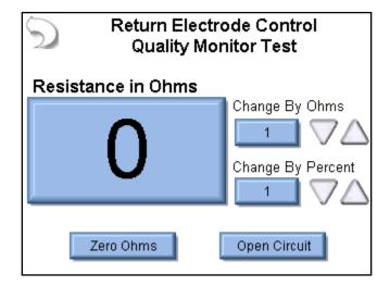
**CQM Resistance** – The CQM resistance can be entered directly be pressing on the resistance indicator button. The maximum CQM resistance is 500 ohms.
