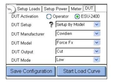
As the load curve runs, the screen will be updated with the measured power from the DUT. At the end of the load curve, there will be buttons available to save the load curve results or view the individual datapoints.
