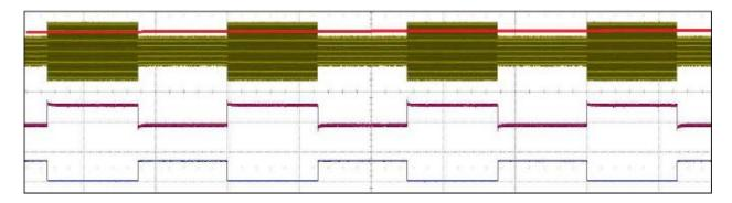
In the above illustration the red line represents the user selectable threshold. The purple signal represents when waveform is above the threshold and the SECULIFE ES PRIME is measuring it as "pulse 1". The blue signal represents when the waveform is below the threshold and is being measured as "pulse 2".
