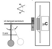
Pendulum damping: by oil filling
