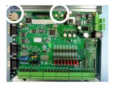
• Insert the LON PCB into the centre of the expansion slot. Please insert with caution and make sure that the all the pins make contact with the appropriate jacks.
