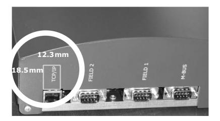
A opening is required in the housing cover of the SMARTCONTROL standard model for connecting the LON plug. Perforations have already been provided for penetration in the housing of models from version 2 onwards.
