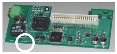
The LON expansion set can only be installed if a basic PCB from revision level 2.3x onwards is available, see encircled marking in the picture below.
