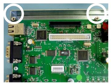
• Fix the LON expansion PCB afterwards with the two M3 screws.
