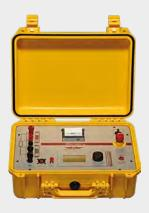
Portable microohmmeter for up to 10 A for testin contact and connection resistance, with a large measuring range of up to 400 k $\Omega$
