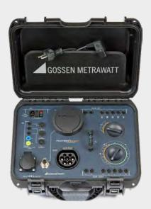
The PROFITEST E-Mobility is an adapter for standards-compliant testing of single and 3-phase, mode 2 and 3 charging cables by simulating faults in accordance with manufacturer specifications. The PROFITEST E-Mobility simplifies your investment decision because quick and safe, standards-compliant testing is made possible for single and 3-phase, mode 2 and 3 charging cables in accordance with manufacturer specifications thanks to accessories which are perfectly matched to the requirements.
