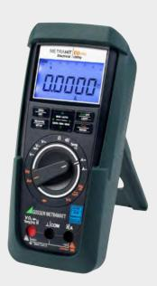
Special multimeter for connection to current transformers without fuses, in order to eliminate danger resulting from interruption of the transformer circuits (and thus measuring category 600 V CAT II)
