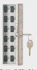
Error Simulator with 12 Error Options via Switches
