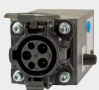
Single-phase test adapter with type 1 plug for testing the effectiveness of protective measures at electric charging stations with the PROFITEST MTECH+ / MXTRA, simulation of fictitiously connected electric vehicles and current-carrying capacity of cord sets per IEC 61851-1
