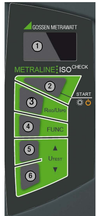
Figure 2.3: Control Panel and OLED Display
