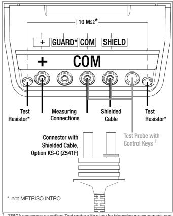
Z550A accessory as option: Test probe with a key for triggering measurement, and an additional key for illuminating the measuring point, including shielded plug-in connector cable
