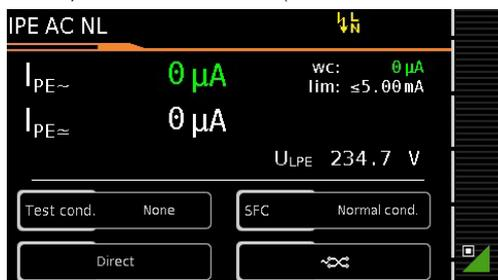
Test Sequence – Test Results (EN 50699 / VDE 0702)
