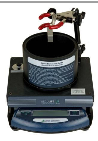
Ultrasound watt meters have been used worldwide since 1977 and are a widely accepted standard for documenting the power output of medical transducers. The Model SECULIFE UP Ultrasound Power Meter was developed to test therapeutic and diagnostic transducers.
