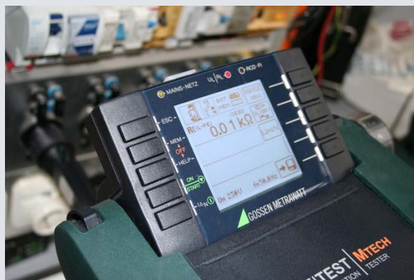
Example of a R E(L-PE) Measurement- 2-Pole measuring with 2-Pole-Adapter
