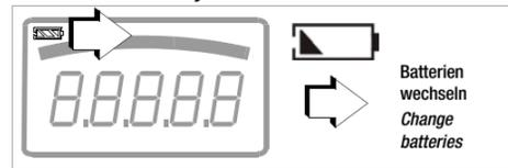
**Batterietausch – Battery Replacement**
