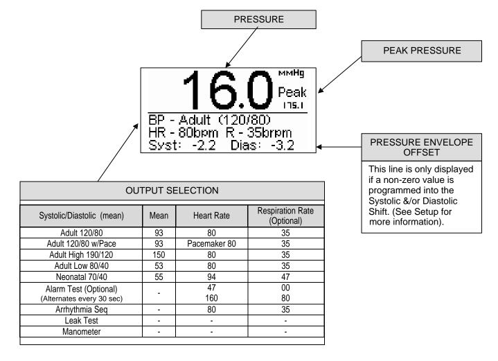
**OUTPUT WAVEFORM SCREEN** – This screen shows the pressure, peak pressure, output selection, and output waveform.
