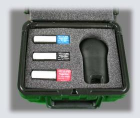
The FingerSim pulsoximeter-testing system enables the user to test pulsoximeters and sensors with three simulated light absorption conditions. These absorption conditions imitate typical oxygen saturations.
