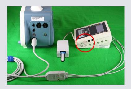
2.) Checking the Sp02 function with the 'SECULIFE pulse oximeter module". The nominal value of the FingerSim<sup>TM</sup> (here: 97 %) should approximately correspond to the value displayed at the DUT (here: 98 %).
