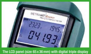
features a background illumination that can be activated, thus creating a clear contrast which facilitates reading, especially in poor lighting conditions.
