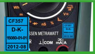
Retraceable evidence and documentation of the technical specification of the device, for example for the monitoring of test equipment in compliance with DIN EN ISO 90000-9004.
