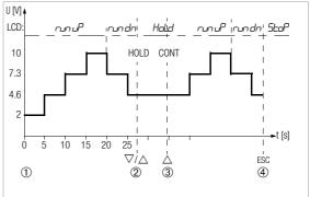
**Interval parameters:** output quantity: U (range of 0 ... 15 V), 5tRrt = 2 V, End = 10 V, number of interval steps = 3, t = 5 s,  $n_{od}E = R_{uto}$
