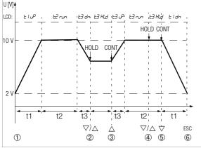
**Ramp parameters:** output quantity: U (range of 0 ... 15 V), 5*L*R-*L* = 2 V, *E*nd = 10 V, *L I* = 5 s, *L*2 = 8 s, *L*3 = 5 s. *rEPERL* for periodic ramp
