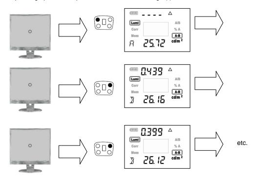
You can switch back and forth between measured values A and B with the MFK.
