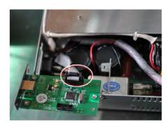
4 Install the interface with the M3 screw (component 3) to the position marked with a white circle in the graph on the right-hand side.
