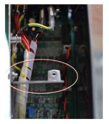
2 Install the connection cable (component 6) in the main board (marked with a white circle in the graph on the right-hand side).
