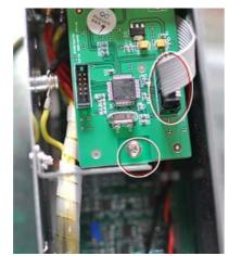
4 Tighten the M4 screws (component 1) at the positions circled in white in the graph on the right-hand side. The installation of the interface is thus completed. Install the housing in the last step.
