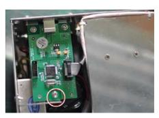
5 Tighten the M4 screws (component 1) at the positions circled in white in the graph on the right-hand side. The installation of the interface is thus completed. Install the housing in the last step.
