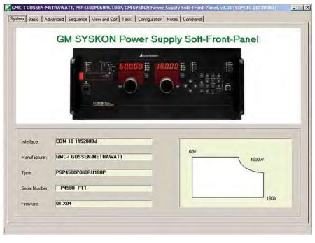
Figure 6: The soft front-panel assures quick, easy operation.
