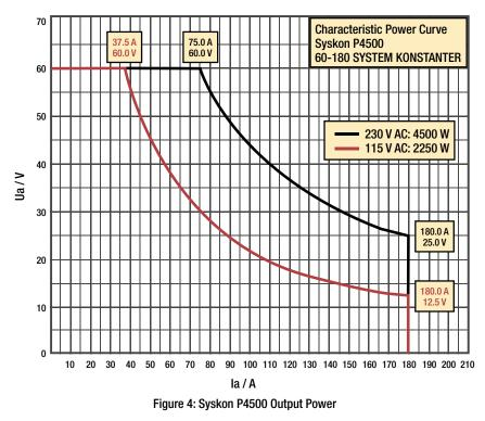
The connection concept for the SYSKON K18000 (figure 5) is implemented by means of a master-slave setup consisting of four SYSKON P4500 devices connected in series via their analog interfaces located in the rear panel. This type of connection allows for output voltages of up to Uset = 240 V and output currents of up to Iset = 75 A. This corresponds to maximum output power of up to Pout = 18,000 W.
