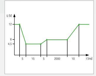
Simulation of a starter motor characteristic curve
