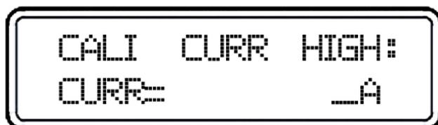
Enter the value you read from the multimeter, which is retained to four decimal places. If necessary, press the "Clear" key to remove the wrong input value of present digit. Then press the "Enter" key to confirm.
