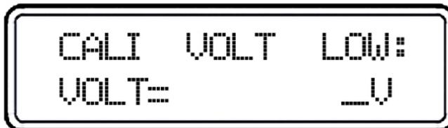
Enter the value you read from the multimeter, which is retained to four decimal places. If necessary, press the "Clear" key to remove the wrong input value of current digit. Then press the "Enter" key to confirm.
