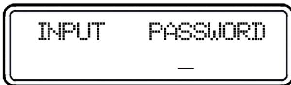
Enter the password "003662", then press "Enter" key to enter into calibration menu, which is shown as below:
