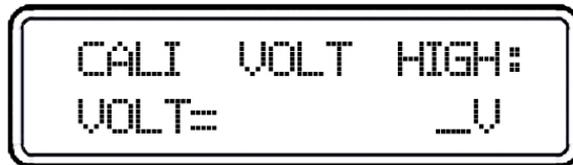
Enter the value you read from the multimeter, which is retained to four decimal places. If necessary, press "Clear" key to remove the wrong input value of current digit. Then press "Enter" key to confirm and exit to calibration menu. Now, voltage calibration is completed.
