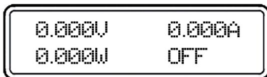
When it is operated from remote interface, entering the following command can enable or disable the output: OUTPUT ON/OFF. You can turn on the output by selecting ON and turn off the output by selecting OFF.
