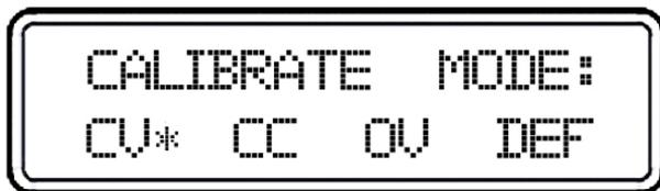
Select CV, CC or OV mode calibration by direction key. If "DEF" is selected, all calibration parameters are restored to default value. CV, CC and OV mode should be calibrated one by one, which is the correct calibration sequence. Return to calibration menu after each mode calibration is completed. Press "Clear" key to exist calibration state.
