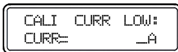
Enter the value you read from the multimeter, which is retained to four decimal places. If necessary, press the "Clear" key to remove the wrong input value of present digit. Then press "Enter" key to confirm.
