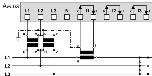
In case of current measurement via L2 or L3 connect voltages according to the following table:
