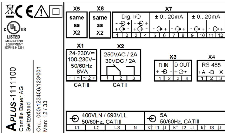
Nameplate of a device equipped with RS485 interface and I/O extension 1
