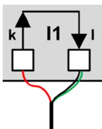
In order to suppress injected interferences the shielding (green) is connected always to the I terminal of the current inputs (I1-I, I2-I resp. I3-I).
