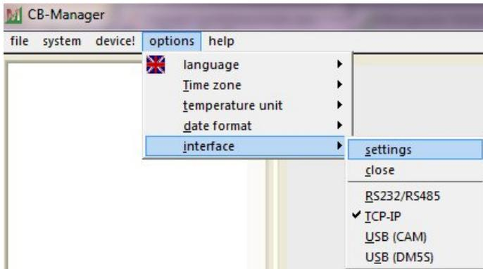
Select "settings" under options | interface. The interface type has to be set to "TCP-IP".
