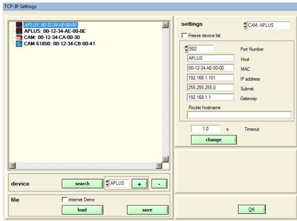
Devices which are not in the same network as the PC (e.g. in the Internet) can not be found and have to be added manually to the device list by means of **+**. The type of the device must be selected previously. To each entry you have to assign a unique IP and MAC address, which are different from the initial value. Otherwise it's not possible to add further entries.
