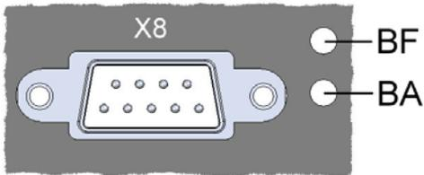
The 9-pin DSUB socket serves the connection of a standard Profibus plug. In a bus terminal device, the bus line must be terminated with resistors in the bus plug. Then standard pin assignment is as follows:
