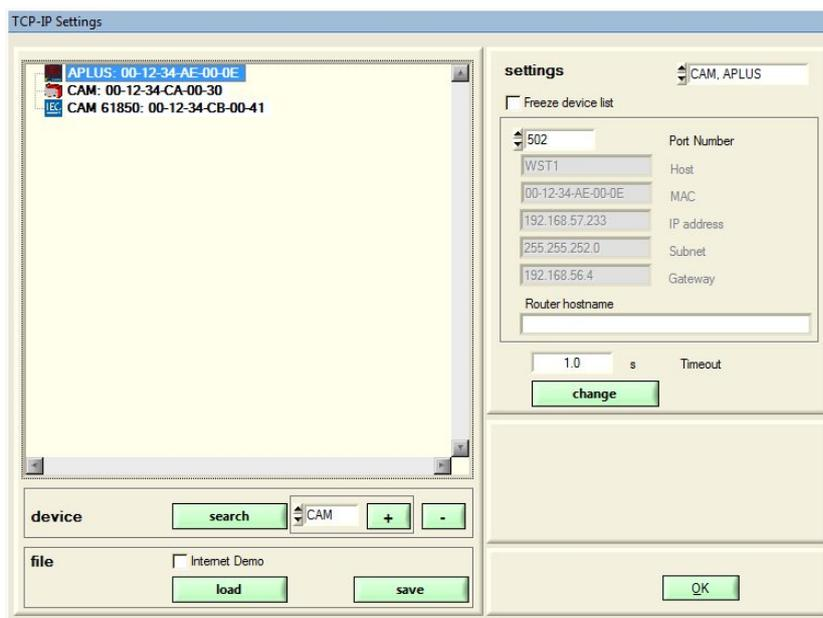
Set settings to "CAM, APLUS". Along with all *APLUS* also SINEAX CAM devices installed in the same network will be shown. The identification of the devices is possible by means of their MAC address, which is given on the nameplate (see [chapter 6.4.1](#)).
