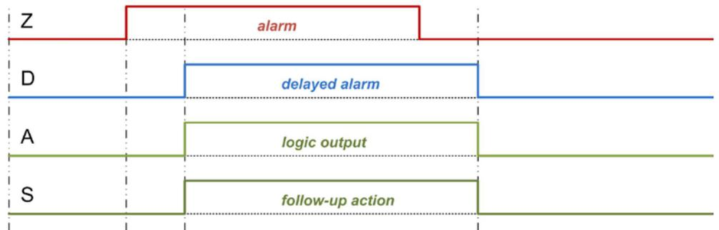
2) Alarm reset active, switch-in and dropout delay 0s, follow-up action inverted
