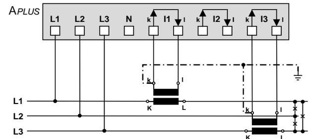
With current and 3 single-pole isolated voltage transformers
