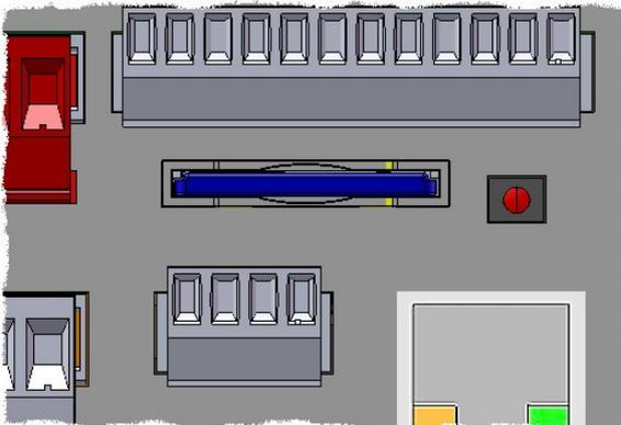
The red LED of the key located next to the SD card signals that the logger is active. During writing to the card the LED becomes dark for a short time.
