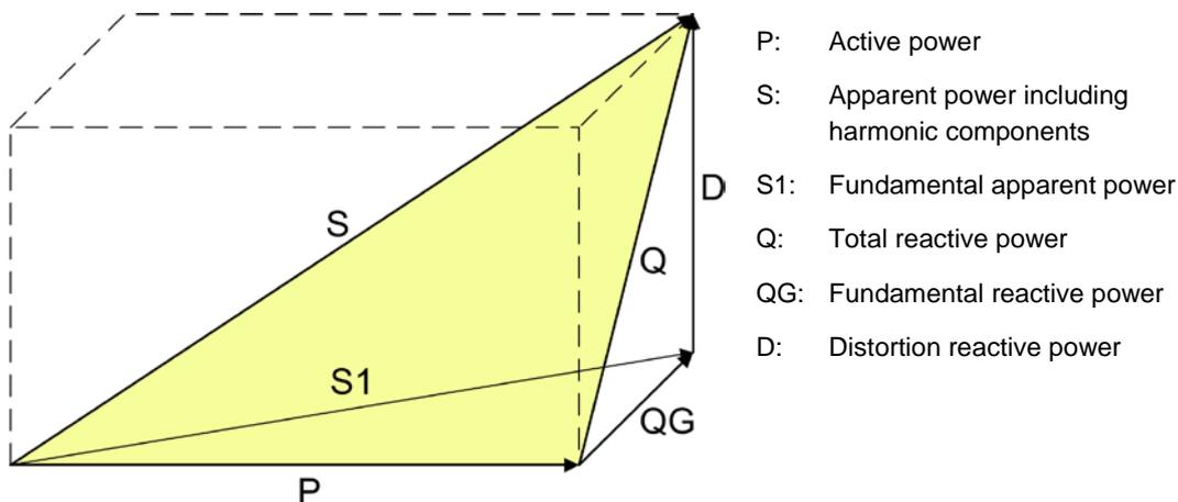
The reactive power may be divided in a fundamental and a distortion component. Only the fundamental reactive power may be compensated directly by means of the classical capacitive method. The distortion components have to be combated using inductors or active harmonic conditioners.
