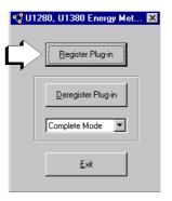
2. Register the plug-in in the installation tool (LONMAKER in this case). After starting LONMAKER, the Plug-In Registration window appears. The plug-in to be registered should appear in the To Be Registered window. Select Finish, in order to register the plug-in.
