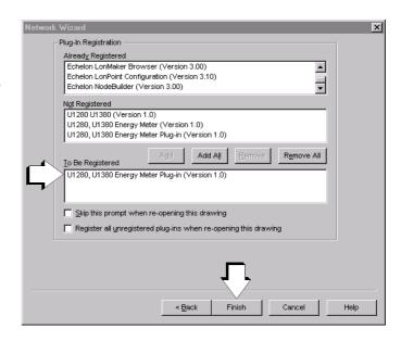
Alternatively, registration can be executed using the Plug-In Registration tab card after clicking Network Properties in the LonMaker menu. Select the plug-in to be registered in the Not Registered window, and click the Add button. The plug-in then appears on the To Be Registered window. Click the OK button.
