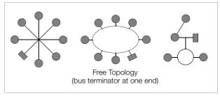
Where bus topologies are used, the individual devices are connected in parallel one after the other. A bus terminating resistor must be used at each end. Only one bus terminator is required with free topologies, but transmission distances are limited in this case.
