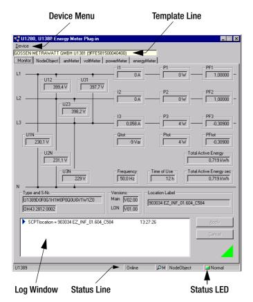
The log window can be cleared or saved to memory with the help of the **Device** menu, and the monitor function can be activated and deactivated.
