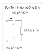
An adjustable bus terminator is frequently included in master stations, which must be set in accordance with the utilized topology. Additional bus terminators are required for bus topologies, and where repeaters are utilized. These can be purchased as auxiliary LON component U1664 in top-hat rail mount housing. Each unit includes a one-ended and a two-ended bus terminator.
